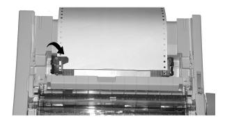
**8** Adjust the position of the right tractor to center the holes in the paper on the pins. Then, close its tractor cover and push back the lock lever. Do not stretch the paper.
