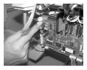
21. Plug the purple cable into the connector on the main board.
