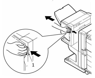
b. Remove the punch collection box from the finisher.
