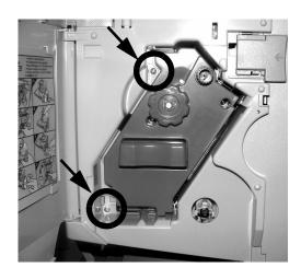
b. Remove the two screws holding the side of the cover in place.
