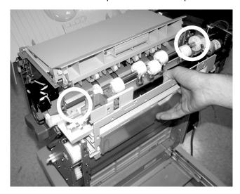
14. Secure the hole punch unit in place: use two of the screws (1) you removed earlier, plus the screw (2) supplied with the hole punch accessory.
