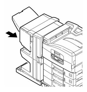
28. Reattach the cable between the finisher and inverter and the finisher power cable.
