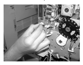
19. Snap open the four cable harnesses, then thread the two cables through the harnesses and snap each one shut.
