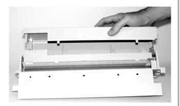
13. Align the pins at either end of the hole punch unit with the holes in the finisher housing, then slide the hole punch unit into place.
