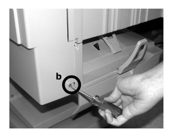
23. Reinstall the internal front cover and secure it with four screws.
