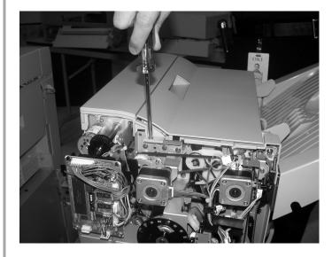
17. Insert the orange cable (4 leads) into the connector on the hole punch unit board.
