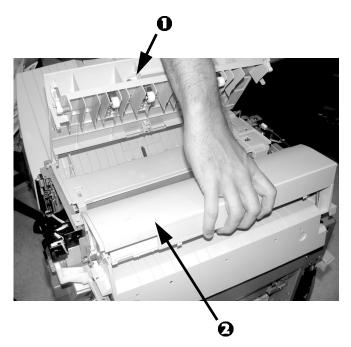
12. Remove the top of the blank unit: you need this to install the hole punch unit. Store the bottom of the blank in case you ever remove the hole punch from the finisher.
