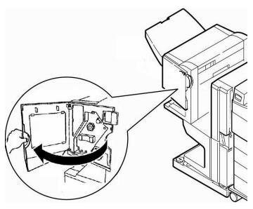
7. Squeeze the white locking tabs on the blue knob and pull it out of the finisher.
