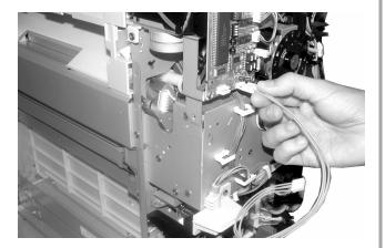
18. Insert the purple cable (5 leads) into the connector on the hole punch unit board.
