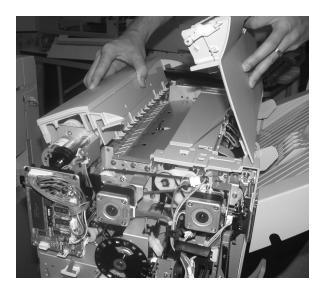
16. Close the top cover and secure the hole punch unit in place with two screws at either end.
