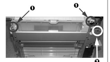
15. Open the finisher top cover and snap the top of the blank into place on the hole punch unit.
