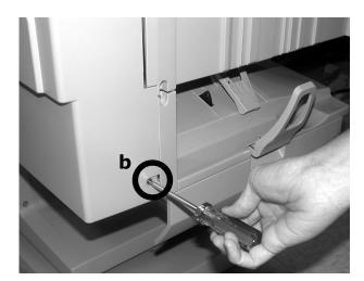
10. Remove the two screws at either end of the hole punch blank.
