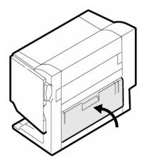
8. Pull the finisher platform about half way out, then loosen the screw on the locking piece (1): viewed from the opposite direction) so that it drops through the slot below it. This keeps the platform from moving while you attach the finisher to it.
