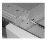
11. Install the stacker, making sure the hooks are firmly engaged and that the lever on the finisher is positioned above the stacker (1).
