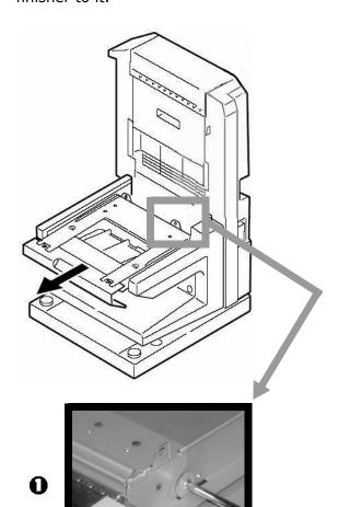
9. Position the finisher on the stand and attach it with two screws from the back.
