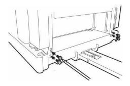
3. Attach the back of the inverter to the stand using one screw on either side.
