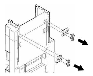
4. Turn the inverter around and remove the two screws holding the extension plate. Keep them handy to reattach the plate once it is repositioned.
