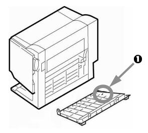
4. Hold the clear band perpendicular to the cover and slip one end over the tab  $(\mathbf{0})$ , then pivot the band 90 degrees (2) so that it is aimed toward the finisher:
