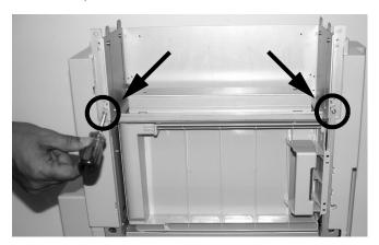
7. Turn the inverter around and reinstall the brackets.
