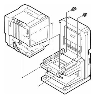
10. Lift the locking piece back up and tighten the screw firmly. Be sure it's out of the way and the screw is tight—otherwise the platform will not move freely.
