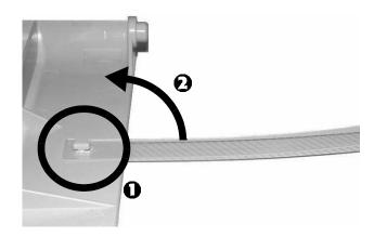
5. Slip the other end of the band (1) through the retainer on the finisher and secure it with the small stopper (2).
