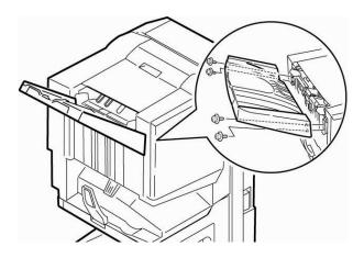
13. Push the finisher against the printer until the prongs on the printer brackets fit into the holes in the finisher.
