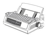
3 Open the access cover. Remove the pull-up roller assembly.
