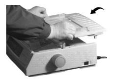
8 Install the pull-up roller assembly. Close the access cover.
