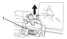
**8** Turn the printhead plate around and reinsert it on the other side of the carriage assembly (1).
