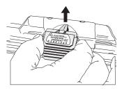
7 Lift the printhead plate off the carriage assembly (1).
