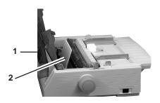
**2** Grasp the tabs and lift off the paper separator (1). Remove the shipping restraint (2).
