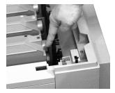
b. Lift the cartridge then slide it toward the back (to clear the tube) and lift it out. Discard it in accordance with local regulations.
