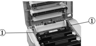
7. Push the two blue retaining levers (1) toward the rear of the printer to lock the fuser in place.
