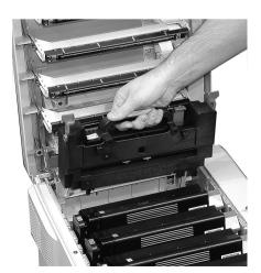
3. Holding the fuser by its handle, lift the fuser out of the printer. If the fuser is still warm, place it on a flat surface which will not be damaged by heat. After letting the fuser cool down, discard it.
