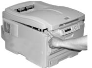
1. Press the cover release and open the printer's top cover fully.
