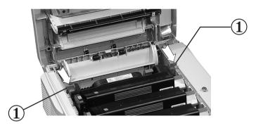
2. Pull the two blue fuser lock levers (1) towards the front of the printer.
