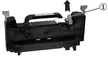
5. Push the orange transport lock (1) to the left to release it (**SNAP!**), then remove the transport lock.
