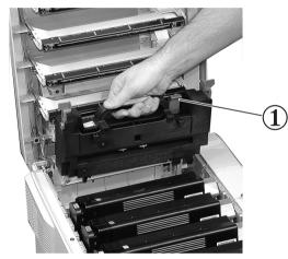
6. Holding the new fuser by the handle, with the fuser pressure release lever (1) on the right, lower the fuser into the priner.
