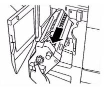
**5.** Turn the knob in the direction indicated to move the stapler to the front.
