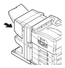
**6.** Operate the Inverter lever (3) and separate the Inverter from the printer.
