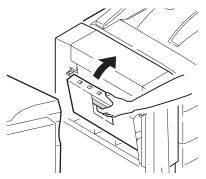
**5.** Move the Finisher back into position and connect it to the Inverter.
