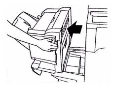
**2.** Pull out the punch chip box, being careful to keep it level so as not to spill any chips.
