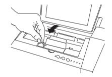
Caution: Ensure that the green Carriage Lock Lever is STILL in the forward position before performing the next step.
