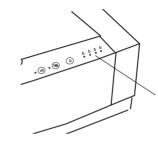
The four Low Ink Indicators are **OFF** when the Colour Print Head is installed and the Ink Cartridges contain ink.
