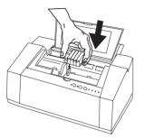
5. Move the green Cartridge Lock Lever backwards to secure the Colour Print Head. Close the Top Cover.
