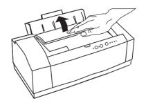
3. Once the Carriage moves to the centre and stops, move the green Cartridge Lock Lever to the forward position and remove the Print Head.
