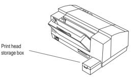
Note: It is strongly recommended that the Print Head be stored in the Storage Box. The Storage Box should be placed in a cool location away from direct sunlight. For best performance, once a month the Print Head should be taken out of the Storage Box, installed in the printer and a few demo prints run before being stored once again, in the Storage Box. WARNING! Keep the Ink Cartridges out of the reach of children. Do not get the ink near your eyes or mouth.
