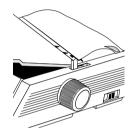
4. Swing the paper separator over, and use the platen knob to draw the quadruple-thick page around the platen: this brings out any jammed bits of paper.
