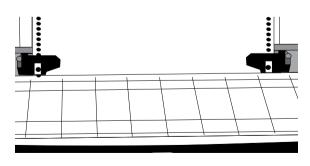
Remove the paper pieces, and use the platen knob to back 7. Replace the pull-up roller assembly, and close the access cover.
