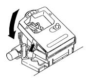
6. Turn the knob (**1**) in the direction of the arrow to take up any ribbon slack.
