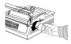
Swing the paper separator over, reload regular paper, and lower the paper separator back into place.
