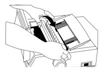
3. Open the access cover and remove the pull-up roller assembly.
