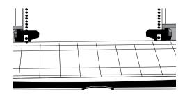
Remove the paper pieces, and use the platen knob to 7. Replace the pull-up roller assembly, and close the access cover.
