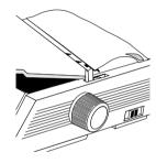
4. Swing the paper separator over, and use the platen knob to draw the quadruple-thick page around the platen: this brings out any jammed bits of paper.
