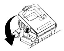
6. Turn the knob (**1**) in the direction of the arrow to take up any ribbon slack.
