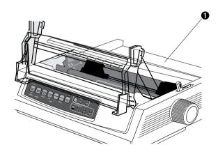
3. Fold some continuous-form paper over three times to make a page four sheets thick, load it on the tractors and close the covers.
