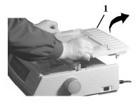
**4** Fold some continuous-form paper over three times to make a page four sheets thick. Then, load it on the tractors and close the covers.
