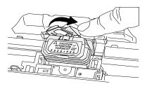
Important! The clamp must be between the black projection on the printhead and the metal plate on the carriage, on both sides.
