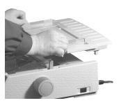
3 Pull up on the lock levers and open the tractor covers.
