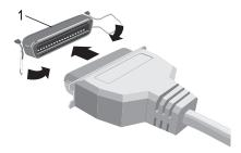
**2** Connect the end containing the standard DB25 connector to the host PCs parallel data port (usually designated as LPT1).
