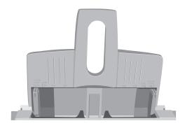
2 Insert the paper so that it is up against and flush with the left paper guide.
