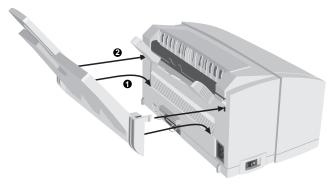
2 Push the paper tray forwards until it latches and is secure on both sides.
