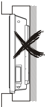
Air circulation is blocked
