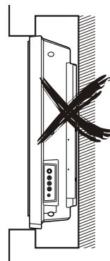
Air circulation is blocked
