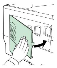
After replacing the toner containers and the waste toner box, clean the main charger units and the paper transfer unit. For instructions, see *Cleaning the Printer on page 3-8*.
