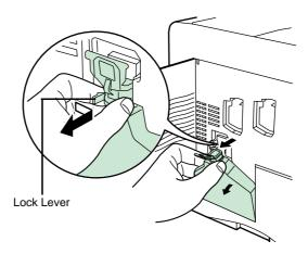
**NOTE:** Remove the waste toner box as gently as possible so as not to scatter the toner inside. Do not let the opening of the waste toner box face downward.
