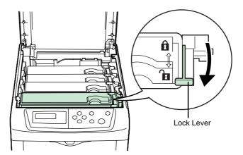
Carefully remove the old toner container from the printer.
