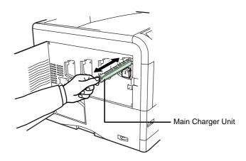
**NOTE:** If the main charger unit is not restored to its home position, the corresponding color will be printed over the whole page.
