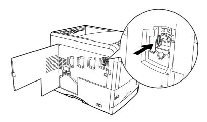
**NOTE:** If the lens cleaner knob is not restored to its home position, the corresponding color will be printed over the whole page.
