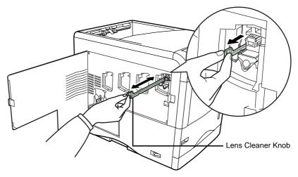
Push the lens cleaner knob back in completely. After cleaning, make sure you restore the lens cleaner knob to its home position.
