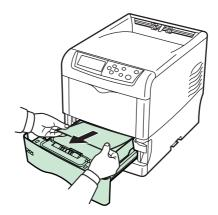
While pulling the green paper transfer unit release lever, pull out the paper transfer unit.
