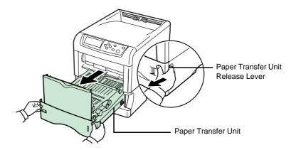
Wipe away the paper dust on the registration roller and the paper ramp using the wiper cloth included in the toner kit.
