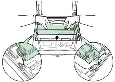
Push down on the top of the toner container to install it firmly in place.
