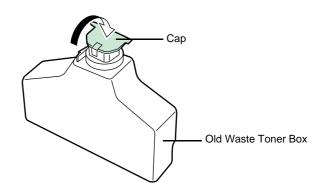
To prevent toner from spilling, put the old waste toner box in the plastic bag (contained in the toner kit) and discard it later according to the local code or regulations for waste disposal.
