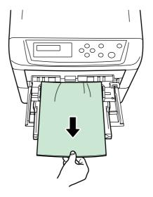
Open and close the paper transfer unit (the paper jam error will be reset).
