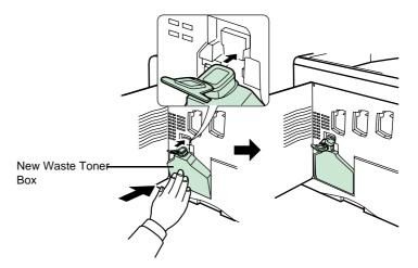
Make sure that the waste toner box is correctly inserted and close the left cover.
