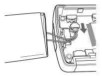
After taking out the battery, tape the cable to the battery body, making sure to cover the connector part, then put the battery in a plastic bag.
