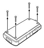
Remove the USB port/RESET button cover, then open the back cover.
