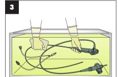
While immersed, detach the adapter from the bronchoscope. Use a clean, lint-free cloth to wipe away any bubbles clinging to external surfaces.
