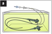
Connect the suction cleaning adapter and syringe. Inject air to remove disinfectant from the instrument/suction channels, then remove the bronchoscope from the disinfectant.
