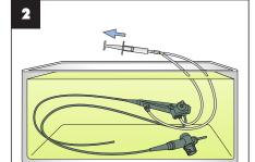
Attach a syringe to the adapter. Pull the plunger of the syringe to fill the instrument/suction channels and channel cleaning adapter with disinfectant solution.
