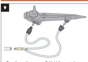
Turn the suction pump off. Hold the control section with the openings pointing down and disconnect the suction cleaning adapter.
