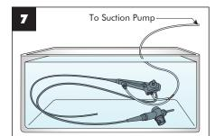
Connect suction cleaning adapter to bronchoscope and to a tube from a suction pump. Aspirate water through channels for 30 seconds. Remove from water and aspirate air through channels for 60 seconds.
