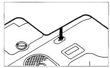
After confirming that the power is ON, press the mid-roll rewind button with the tip of a ballpoint pen, or the like. Do not use an instrument with a sharp tip.
