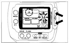
Note: If the shutter speed indicator blinks, adjust the aperture until the shutter speed lights steadily.
