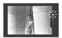
Make sure) The autofocus beep is heard and the autofocus indicator lights when the subject is in focus. It will blink if the subject is difficult for the autofocus to lock on, and when the subject is too close. Note: When the autofocus indicator blinks, the shutter won't release. (See p. 70.)
