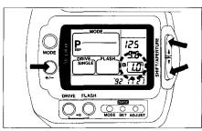
(Make sure) The exposure level is displayed in the viewfinder and on the LCD panel.
