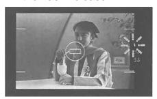
When the flash is flipped up, the camera will start recharging the flash.
