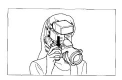
Note: When used together, the G40 fires full emission but the built-in flash is compensated by -3EV.
