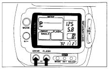
When overriding or reactivating the beep, a confirmation beep is heard. Note: When the power is switched off and on again, the beep will be functioning.
