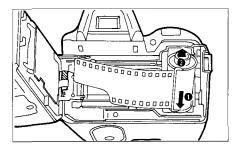
Note: Use DX-coded film. Caution: Do not touch the shutter curtain, and do not press it with the edge of film.
