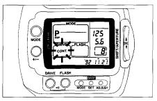
**L** button is fully pressed, the shutter releases continuously.
