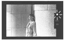
Note: When there is no subject in the position you want to focus on, first focus on an object at the same distance as the desired position. Then enter the PF mode, and recompose the frame. (See page 52.)
