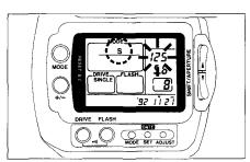
Note: If the aperture indicator blinks, adjust the shutter speed until the aperture indicator lights steadily.
