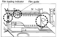
Note: Make sure the film is lying flat. If not, push the cartridge down.
