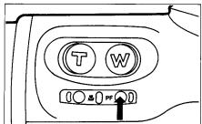
Note: Manual focusing is possible using the zoom buttons, but zooming cannot be performed in the PF mode. To cancel the PF mode, press the PF button again.
