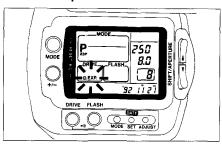
2. Press the shutter release button fully to take the first exposure.
