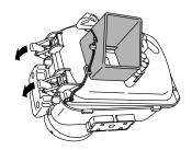
▲ CAUTION: • Seal the Case by turning both buckle lock levers down in arrow direction. When one of the buckles is left open, the Case will not be sealed and water leakage will be caused.
