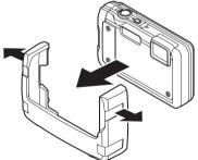
White adapter (PTAC-06) for  $\mu$  TOUGH-6020/STYLUS TOUGH-6020. Black adapter (PTAC-07) for  $\mu$  TOUGH-8010/STYLUS TOUGH-8010.
