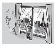
Move to a location where the signal can be easily received. Inside a building, broadcast signals will be more easily received near windows.
