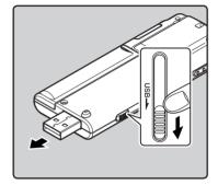
3 Make sure that the recorder is stopped, and connect to the PC's USB port.
