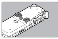
Face the card the correct way and insert it into the card slot as shown in the diagram.
