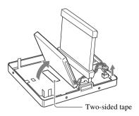
**6** Tape the cable to the battery body, and put the battery in a plastic bag, etc. Cover the connector with tape before you put the battery in a plastic bag.
