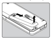
Insert the battery, observing the ⊕ and ⊖ polarities.
