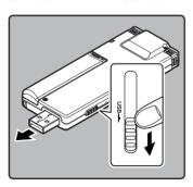
3 While pressing the STOP (■) button, connect to the PC's USB port.
