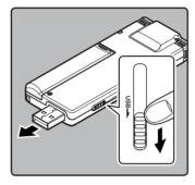
3 Connect to the PC's USB port or to a USB hub.
