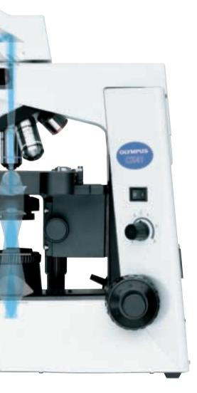
Phase-contrast condenser / CX-PCD The multi-purpose CX-PCD condenser allows observation of brightfield, phasecontrast and darkfield images without
