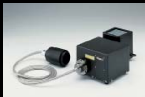
Transmitted Light Detection Unit External transmitted light photomultiplier detector and 100 W Halogen conventional illumination, integrated for both laser scanning and conventional transmitted light Nomarski DIC observation. Motorized exchange between transmitted light illumination and laser detection. Simultaneous multi-channel confocal fluorescence image and transmitted DIC acquisition enabled.
