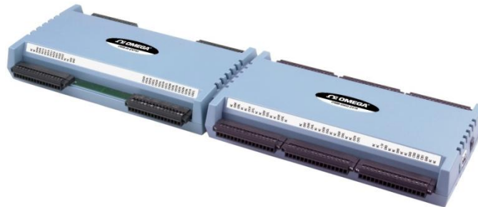
Figure 1. OMB-DAQ-2416-4AO directly connected to an OMB-AI-EXP32
