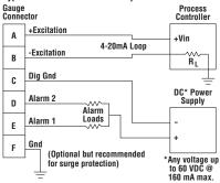
$R_L = 250$  ohm for 1-5 V output  $R_L = 500$  ohm for 2-10 V output
