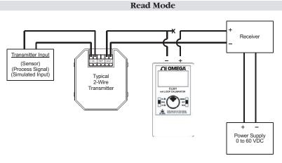
The CL531 can read loop currents from 0-24 mA. The CL531 limits current in read mode to 25mA to protect the devices in the loop from over voltage or over current conditions.
