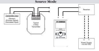
Source mode uses internal power to supply current from 0.00-24.00 mA into as much as  $1200\Omega$  until the end of battery life. The calibrator Graph will flash if connected improperly. The three-position EZ-Check switch provides instant preset 4mA at zero, 12mA at mid range and 20mA at full scale outputs. The output is adjusted in 0.01 or 0.10 mA increments (0.1 or 1.0) % display units with the EZ-Dial knob.
