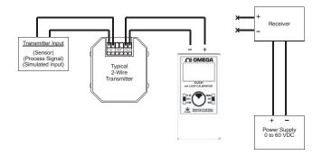
The CL531 supplies 15Volts or 24 Volts to the transmitter and displays the output in mA or % on the CL531 display. In read mode press the EZ-Dial™ Knob twice to get into the feature options. Then press the EZ-Dial™ Knob to select mA PWR - M. Then turn EZ-Dial™ Knob to select power range (15V or 24V). The EZ-Check switch and EZ-Dial knob allow rapid and fine control of loop current.
