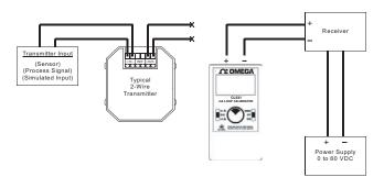
The CL531 can simulate a 2-wire transmitter in the 4-20 mA or % process loop. In source mode press the EZ-Dial™ Knob twice to get into the feature options. Then press the EZ-Dial™ Knob to select mA 2 – wire. The EZ-Check switch and EZ-Dial knob allow rapid and fine control of loop current.
