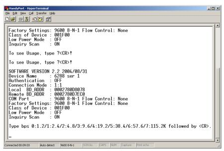
Type '7' (for the baud rate 115200) and press the *Enter* Key.
