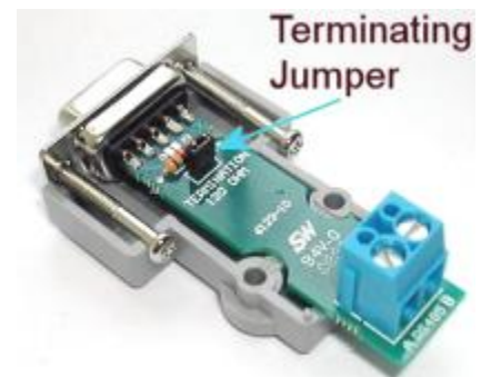
Fig 3-19 RS485 120 Ohm Jumper
