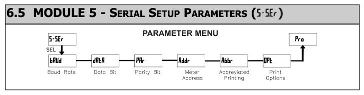
The Serial Setup Parameters are only active when the optional RS232 or RS485 serial communications module is installed in the meter. Refer to the DP6-COM bulletin for complete details on DP63000 serial communications.
