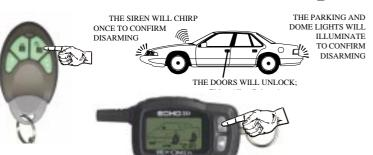
\*An optional doorlock interface, in either standard form or driver's door priority form, must be installed
