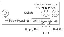
the sensor while calibrating because this will cause a false reading. Using a small nonmetallic screwdriver or alignment tool, turn trimpot Full until the LED just lights, and no farther. Note the position. Now turn the trimpot back until the LED turns off. The ideal setting for the trimpot is midway between these on and off points.
