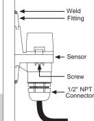
adhesive provides a seal between the sensor and the tank wall, and will hold it in place during testing and installation. If desired, the sensor may be installed temporarily without weld-
