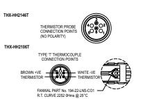
WARNING - Do not bring probe into contact with any service connected to a hazardous voltage (i.e. a voltage exceeding 30 volts RMS or 42.4 volts peak with respect to either earth or ground). Ensure that the probe is suitable for the application, paying particular attention to the temperature range and type of thermocouple. Connect probe plug into the socket at top of instrument. NOTE: Only probe listed should be used with the HH2100 series thermometer range.
