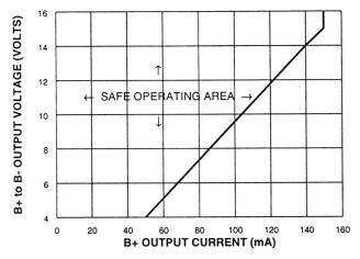
**NOTE:** To operate safely in the "unsafe" area of the curve, at low voltage settings, use an external resistor in the B+ line, to take most of the drop externally, and connect the + sense line in the normal manner. Do not allow prolonged shorts across the output.
