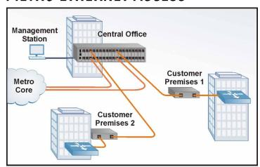
At the Central Office, the 2GXM2 plug-in module is installed in a managed *iConverter* 19-Module chassis providing high-density fiber access. At Customer Premises 1 and 2, the 2GXM2 standalone NID provides a fiber uplink port for intelligent demarcation of Ethernet services.
