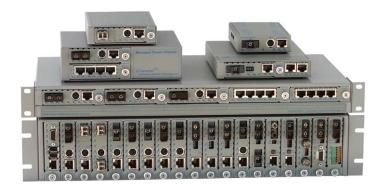
*iConverter* 4Tx modules are hot-swappable and can be mounted in a 19-Module (2U high) or 5-Module (1U high) rack-mountable chassis (19-inch or 23-inch) with any combination of redundant AC, 24VDC or 48VDC power supplies. They can also be mounted in a 2-Module AC or 18 to 60VDC powered chassis, or in a 1-Module AC/DC powered chassis.
