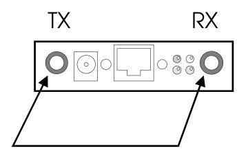
To test the integrity of copper patch cables and any intervening baluns connect the OmniHawk<sup>™</sup> to an unused lobe of any powered hub. If the cable is unbroken, the copper ready LED will light green. If the cable is broken, the LED will be off.
