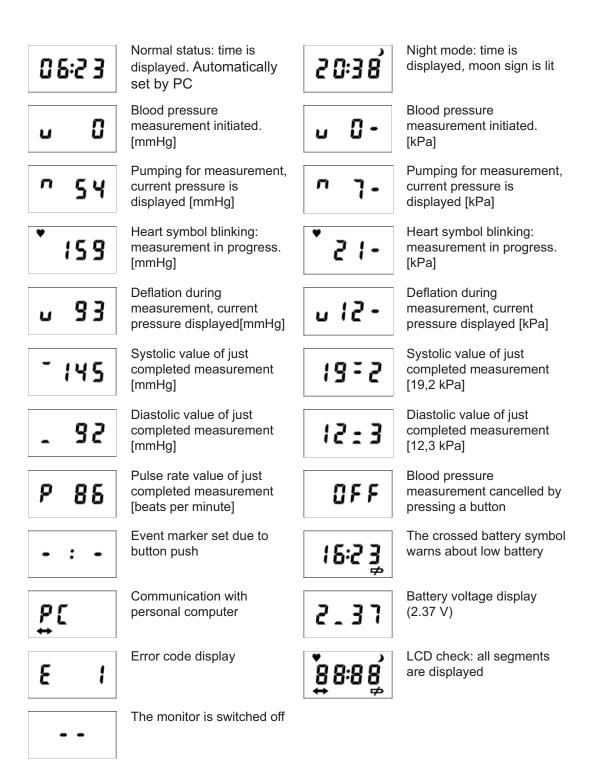
The monitor must be programmed with the **OMRON BP Tracker Software** installed on the computer (for details see Software Manual). Once the preprogrammed time is reached, the monitor will start operating automatically and perform blood pressure measurements based on the monitoring plan. To obtain reliable BP readings, certain rules must be observed.
