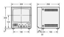
ALL DIMENSIONS SHOWN ARE IN MILLIMETERS. To convert millimeters into inches, multiply by 0.03937. To convert grams into ounces, multiply by 0.03527.
