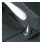
Cleaning the discharger electrodes
