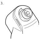
The horn can be cleaned with vinegar. Moisten a cloth with vinegar for surface cleaning. Mix one part vinegar and three parts distilled water to be run through for 45-60 seconds for internal horn cleaning.
