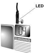
Test the *Home Producer*. The Command Center will convert the RF signal from the Home Producer into an IR signal and transmit that signal to your component through the IR signal extension cord.
