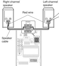
• To prevent damage to circuits, never short-circuit the positive (+) and negative (-) speaker wires.
