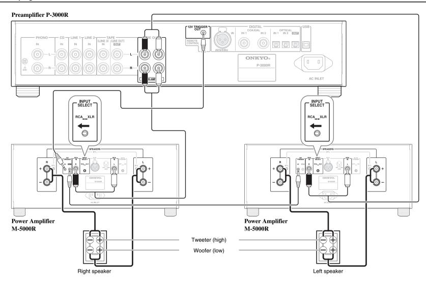
This is an example of the bi-amping connection using the preamplifier P-3000R.
