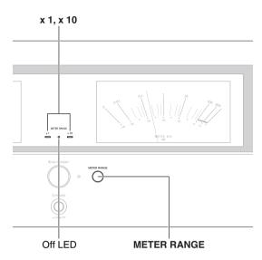
You can switch the power output of speaker terminals between **×1** (default) and **×10** (10 times).
