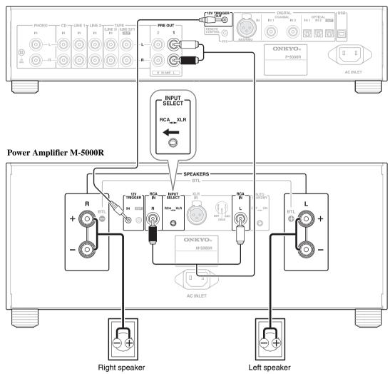
This is an example of the stereo connection using the preamplifier P-3000R.
