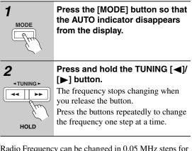
Radio Frequency can be changed in 0.05 MHz steps for FM and 9 kHz steps for AM. You can change the interval of the steps for AM frequency (not European models) (see page 55).
