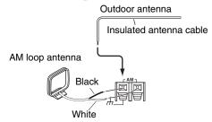
Outdoor AM antennas work best when installed outside horizontally, but good results can sometimes be obtained indoors by mounting horizontally above a window. Note that the AM loop antenna should be left connected. Outdoor antenna must be grounded in accordance with local regulations to prevent electrical shock hazards.
