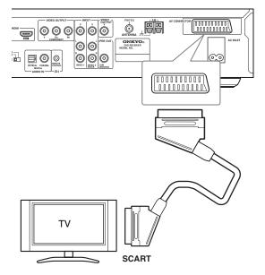
This connector can output composite video, or RGB video. The default setting is composite, which should work with all TVs. Consult the manual that came with your TV to see if you can use one of the higher quality settings. See page 62 for how to change the video output.
