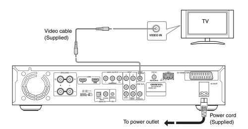
This receiver is equipped with copy protection technology. Do not connect this receiver to your TV via a VCR using Video cable, as the picture from this receiver will not appear properly on your TV. (This receiver may also not be compatible with some combination TV/VCRs for the same reason; refer to the manufacturer for more information.)
