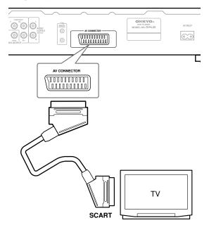
This connector can output composite video, S-Video, or RGB video. The default setting is composite, which should work with all TVs. Consult the manual that came with your TV to see if you can use one of the higher quality settings. See page 41 for how to change the video output.
