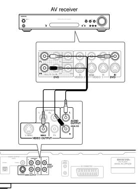
The diagram shows standard video connections, but you can alternatively use the S-Video or component video connections if they're available.
