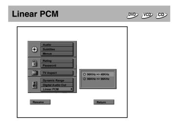
**96KHz**  $\Rightarrow$  **48KHz:** Even in case of 96 kHz digital signal, the DVD player will deliver 48 kHz signal out.
